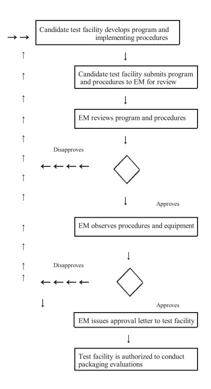
Figure IV.2. Procedural steps for establishing a Type A test program at a test facility.
