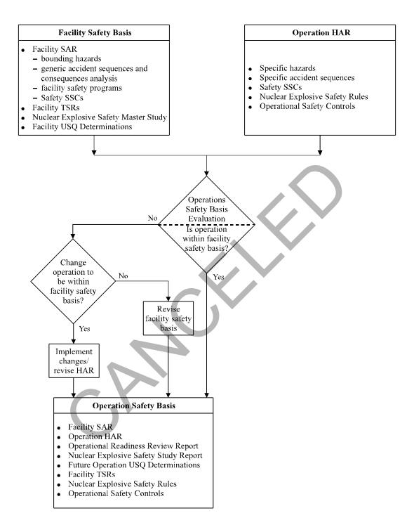
Figure 1. Safety Basis of a Nuclear Explosive Operation
